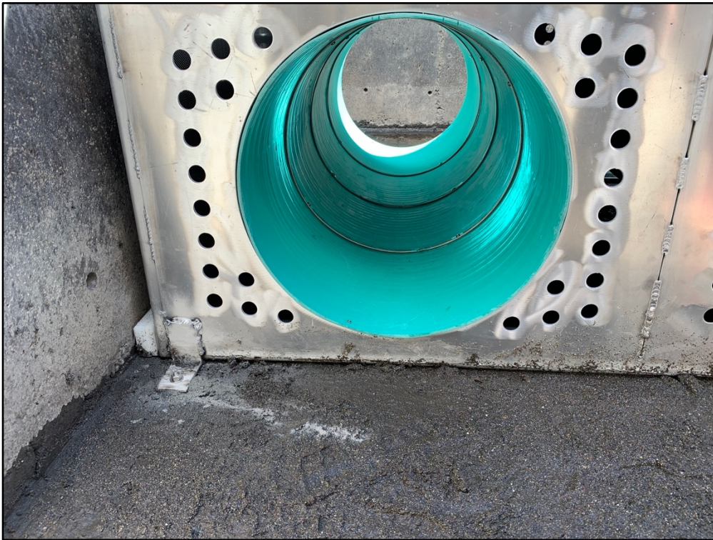
Figure 3-3. View through a resistivity-type fish counter (photo credit: Frank Edgson).
